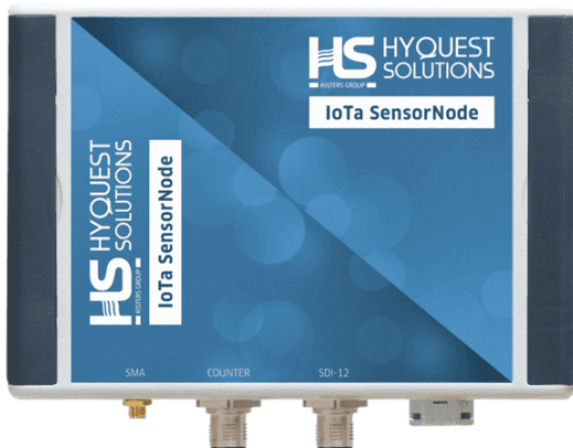
Figure 1 - IoTa SensorNode in portrait view with labelled connectors at the bottom
