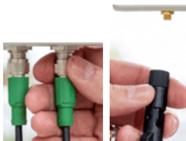
Figure 2 - Connecting a signal cable(left) and the antenna (right)
