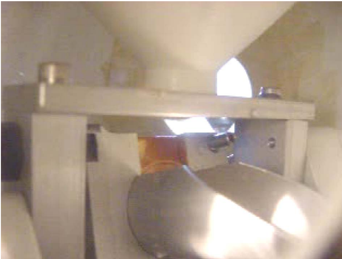
Figure 56: Photographs of the h-340SDI sensor showing water droplets being pulled sideward and missing the tipping bucket when the sensor is internally wet.
